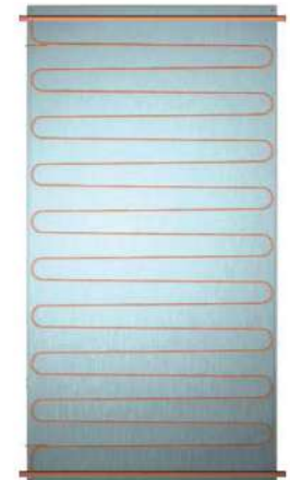
Meander collector with manifolds (MS) with up to 10 collectors in parallel connection, low-flow up to 15 collectors.
