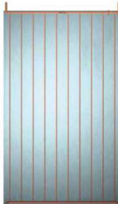
Double-harp collector (DH) with up to 6 collectors in series connection, low-flow up to 8.
